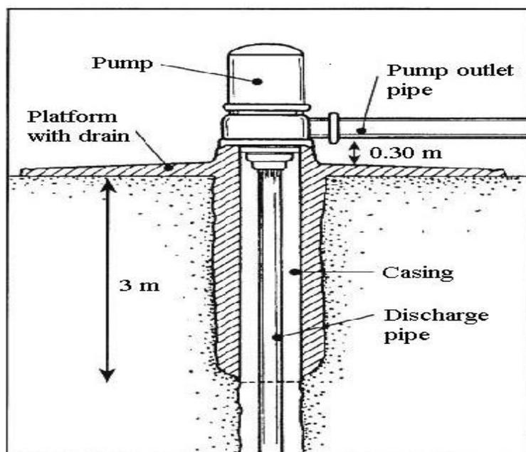
Fig. 2 : Schematic representation of an improved deep well
