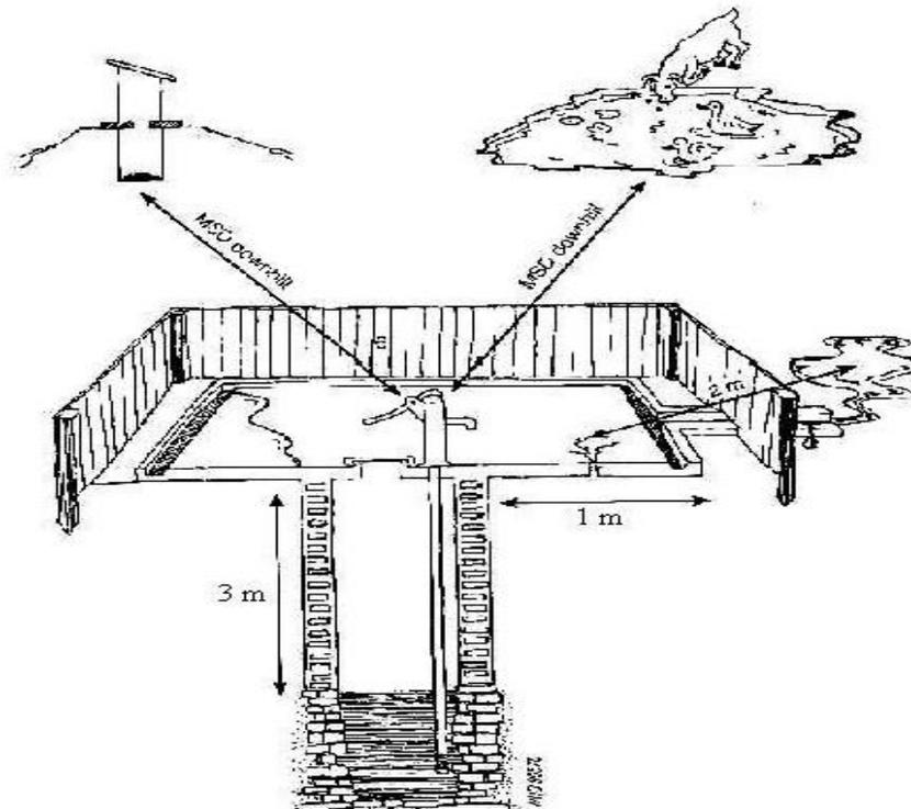
**Fig. 1 :** Sources of the contamination within the well boundary
