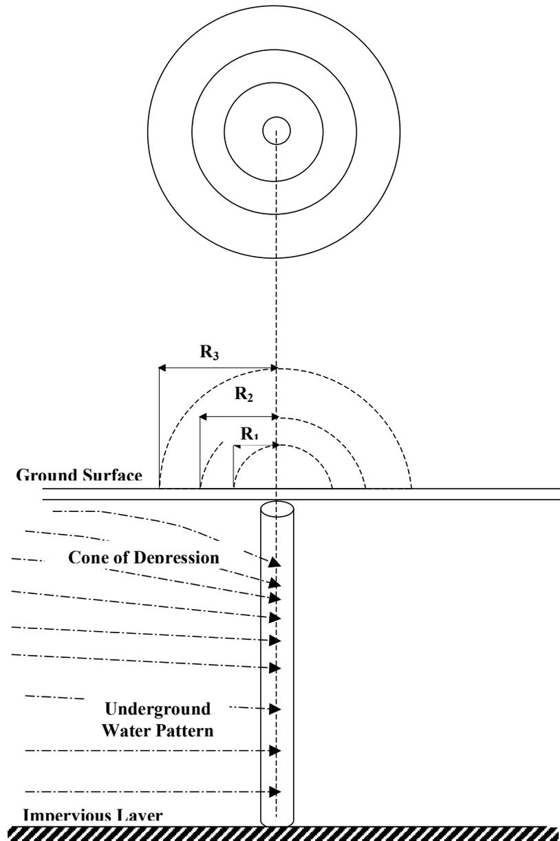
Fig. 4 : Hydraulic characteristics of different types of the sanitary boundaries
