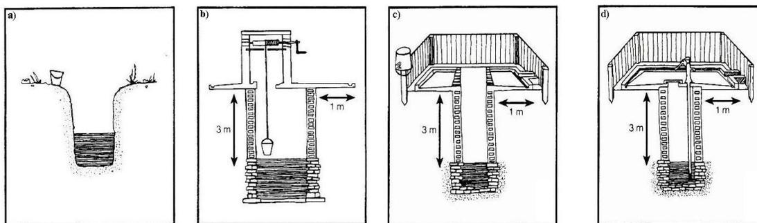
Fig. 3 : Schematic representations of the wells : (a). Dug well, (b). Dug well with wheel, (c). Uncovered dug well and (d). Improved well with back hand pump
