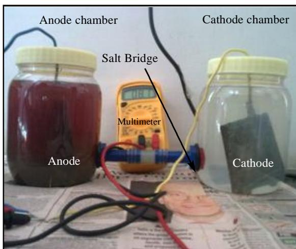
Fig. 1: Assembly of MFC used in present studies
