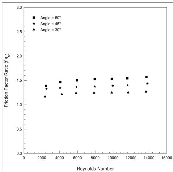
**Fig. 4 :** Friction factor ratio versus Reynolds Number
