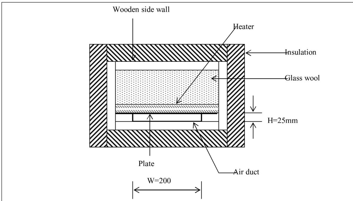
Fig. 2 : Cross-sectional view of experimental set up
