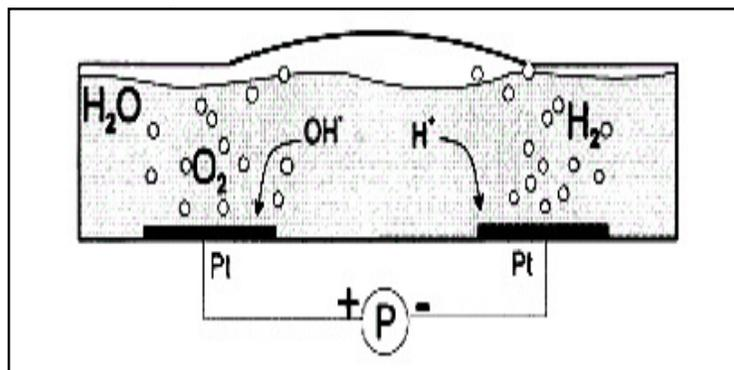
**Fig. 1 :** Sketch of an electrochemical cell
