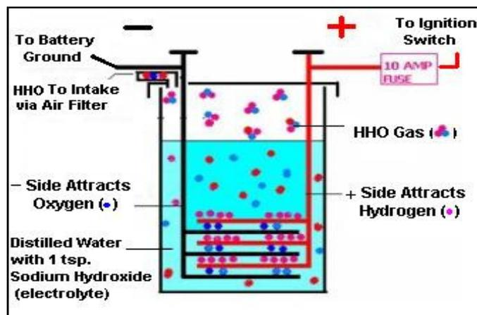
Fig. 2 : Alkaline water electrolysis
