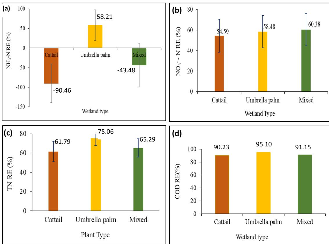
**Fig. 3 :** The average removal efficiencies of (a)  $\text{NH}_3\text{-N}$ , (b)  $\text{NO}_3\text{-N}$ , (c) TN and (d) COD, in cattail, umbrella palm and mixed vegetation wetland units over the study period
